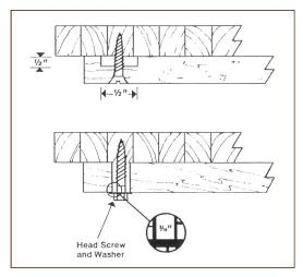
Some manufacturers of cabinets and appliances take into consideration expansion and contraction by providing slotted screw holes. Locate the screws in the center of the slots. Where a manufacturer has not made such allowances, use an undersized screw with a washer. A suggested way to make this allowance in attaching wood parts is to counter sink the pilot holes where the wood part attaches to block, or make the pilot holes oversized using a flat head screw and a washer.
